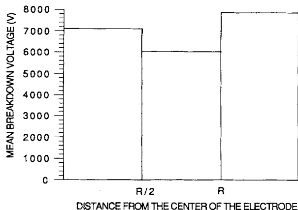
Figure 2 Mean breakdown voltage of an aged PP film in concentric rings, at different distances from the center of the electrode.
